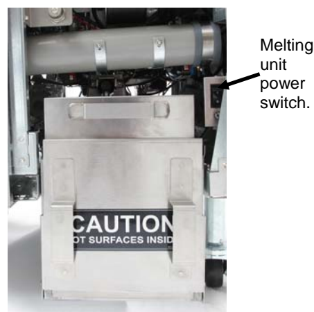
Figure 8: The assembled melting unit is shown in position.
