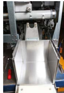
Figure 1: Position melting unit in front of cabinet.
